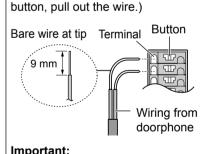
Do not connect the power cable. (Damage may occur.)
