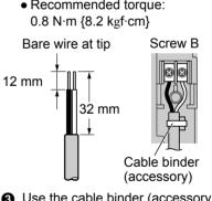
Use the cable binder (accessory) to secure the DC cable (double-coated area) to the main monitor.
